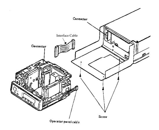
Figure 1-24. Attach the ACL Mechanism
